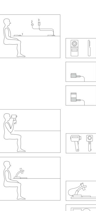
Measuring horizontal illuminance on the working plane using measuring equipment with an integral photo-cell (1).
